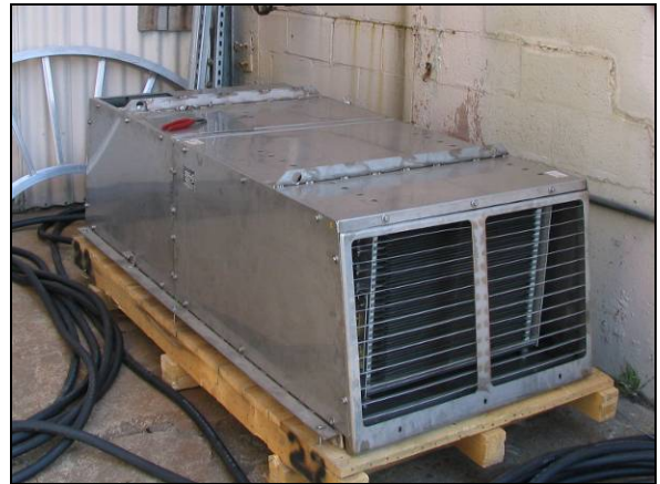
Figure 8. Locomotive braking resistor being installed for loading up to 1.3 MW
