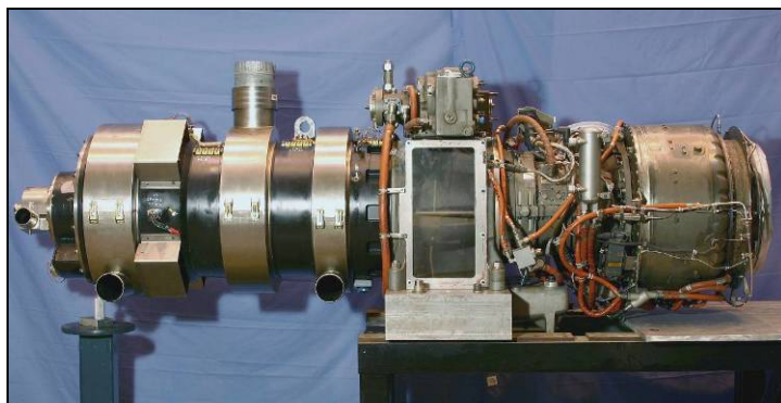
Figure 2. ALPS HS-Generator mounted with a Navy TF40B engine (1700 kg, as shown)
