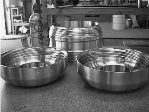
Figure 1. Containment shroud and end plates.
