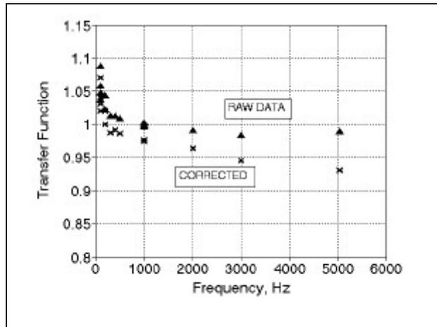
Figure 3. Probe A Sine Wave Gain Data, Raw and Corrected.
