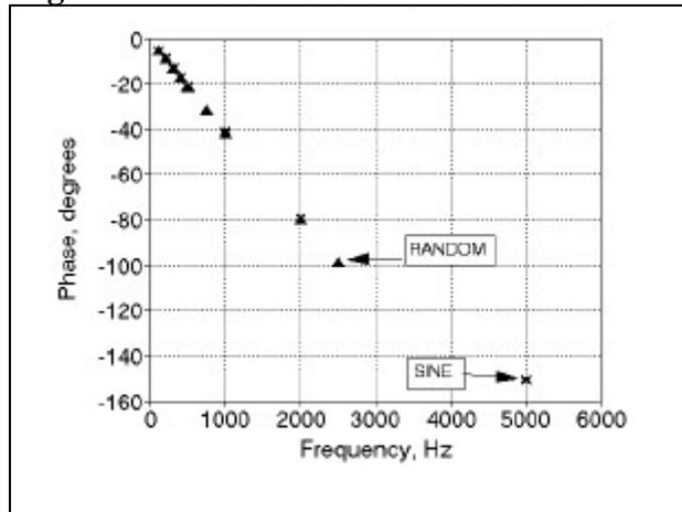
**Figure 11. Probe B Corrected Phase Data, Sine and White Noise.**
