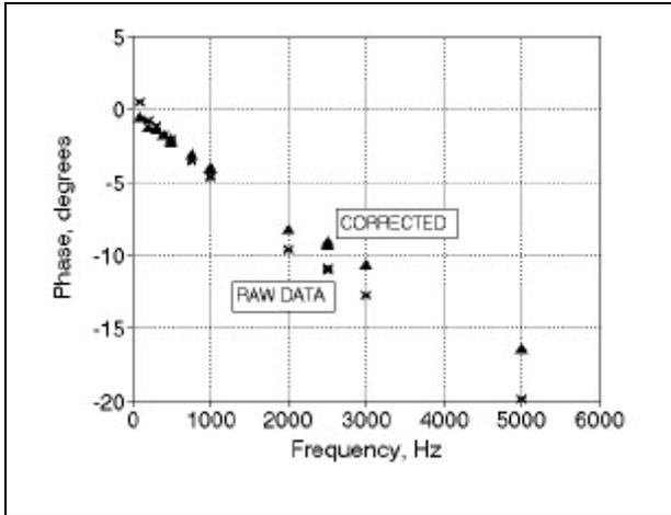
**Figure 6. Probe A White Noise Phase Data, Raw and Corrected.**
