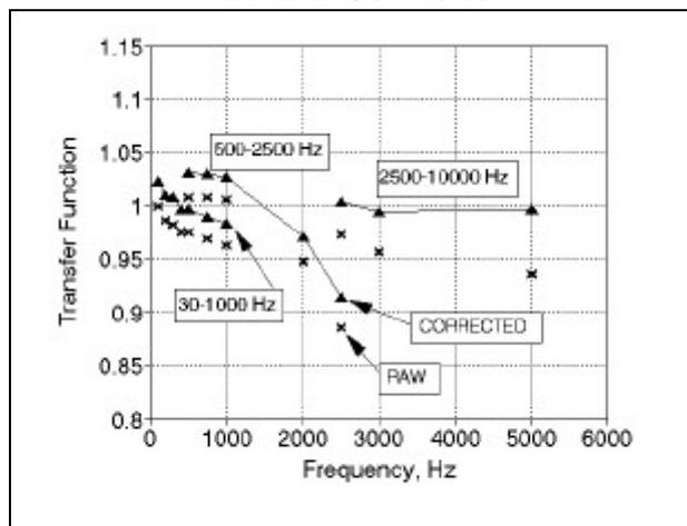
Figure 5. Probe A White Noise Gain Data, Raw and Corrected.
