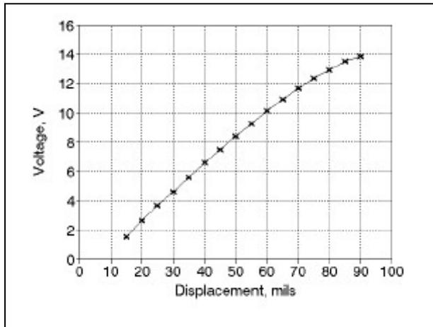
Figure 2. Probe A Static Calibration Curve.
