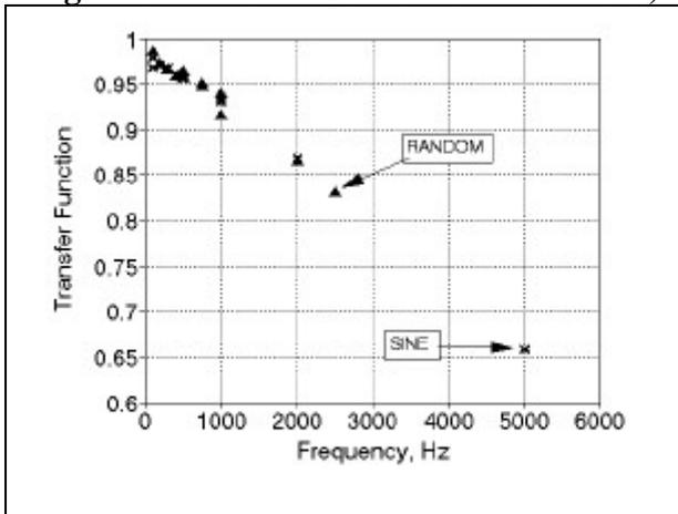
**Figure 10. Probe B Corrected Gain Data, Sine and White Noise.**
