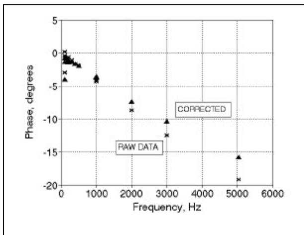
Figure 4. Probe A Sine Wave Phase Data, Raw and Corrected.
