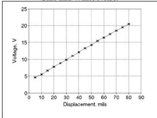
**Figure 9. Probe B Static Calibration Curve.**
