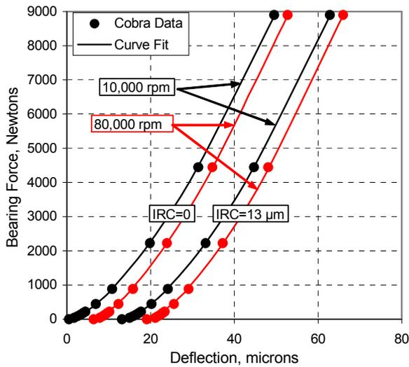
**Figure 3:** Load vs deflection for ball bearing.
