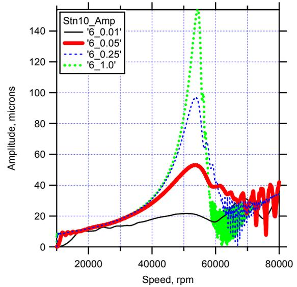
**Figure 5:** Speed ramp data for 6  $\mu\text{m}$  IRC.
