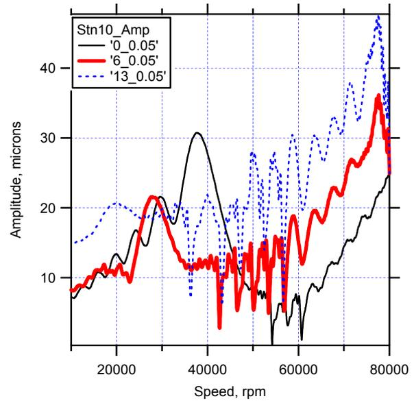
**Figure 12:** Deceleration data for 0.05 sec. ramp time.
