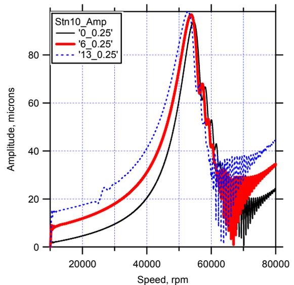
**Figure 8:** Acceleration data for 0.25 sec. speed ramp.
