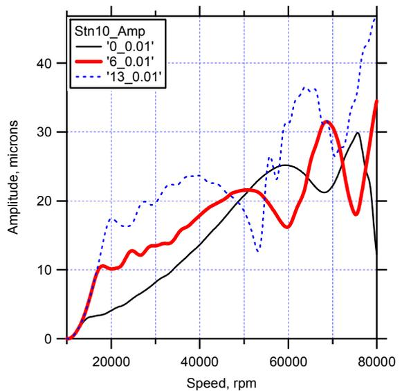
**Figure 10:** Acceleration data for 0.01 sec. speed ramp.
