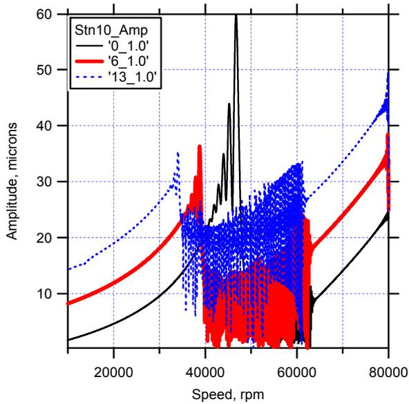
**Figure 11:** Deceleration data for 1 sec. ramp time.
