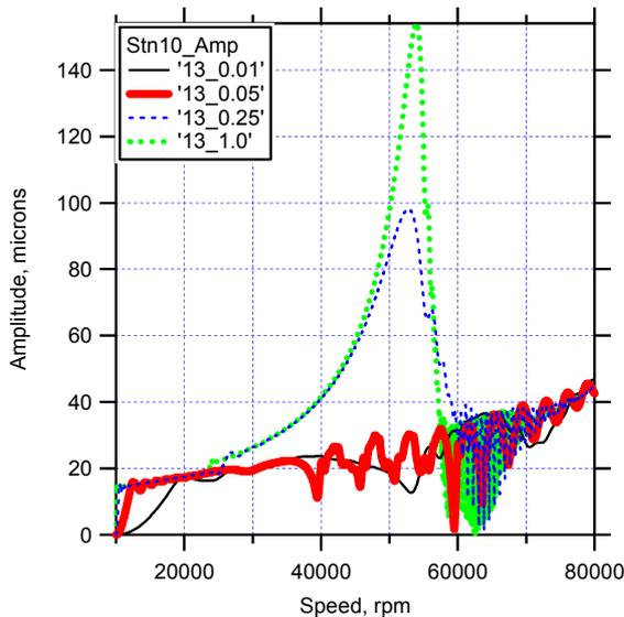
**Figure 6:** Speed ramp data for 13  $\mu\text{m}$  IRC.
