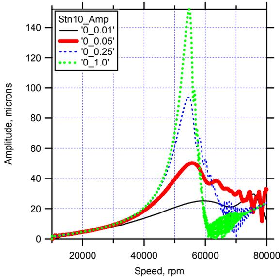
**Figure 4:** Speed ramp data with zero IRC.
